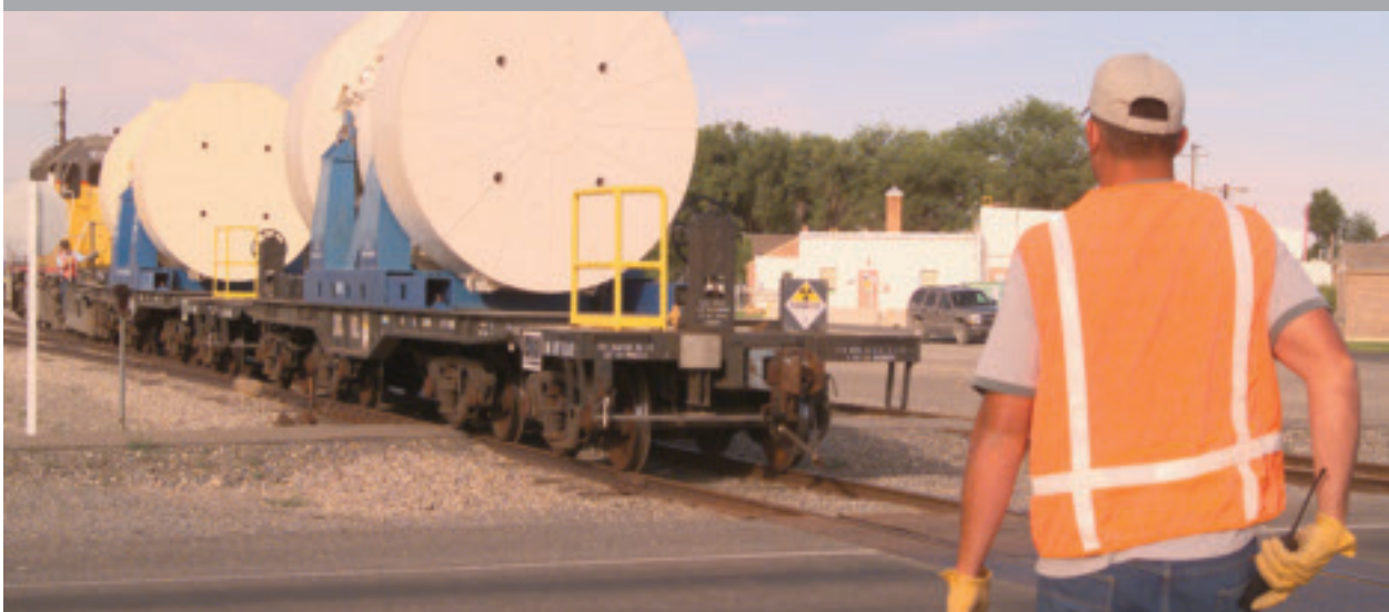
FIGURE 19. CASKS BEING TRANSPORTED BY RAIL
